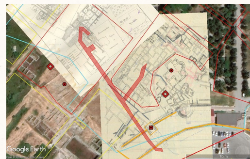
The trench 2024 for laying utility lines (in red), block boundaries (yellow and red lines) and archaeological plans based on the results of excavations of the 19th–20th centuries.
